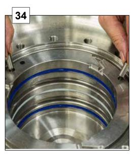
To make the reassembly of the motor easier, make a mark on the outside of the stator frame where the holes for the dowel pins are positioned.
