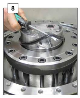
Remove 15 pcs M12x110 screws to loosen the motor part.
