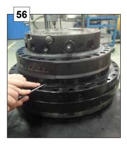
Dry the surface of the slewing bearing clean with paper. Clean the seal groove.
