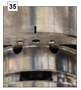
Make a mark inside stator upper where the dowel pins are assembled.
