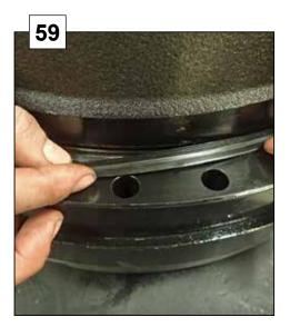
Make sure that the seal gets into the groove on the slewing bearing correctly. Assembly can be made by hand.
