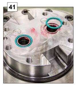
Torque the screws 120 Nm.
