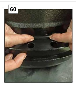
Inspect that all parts of the seal is seated in the groove on the whole round.
