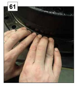
Correct positioned seal.
