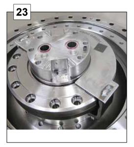
Disassemble the plugs/fittings from the grapple- and rotation inlets. That will make it easier to lift the motor off.
