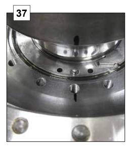
Assemble the motor by knocking it down carefully with a plastic mallet.
