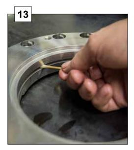
Assemble a new seal in stator lower.
