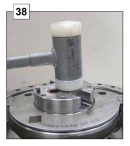
Assemble 15 pcs M12x110 screws. Crosswise tightening.
