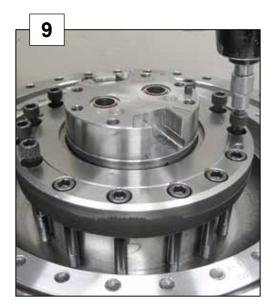
10 Disassemble the stator lower by carefully bending from
