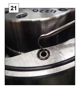
Assemble stator lower on the motor part.
