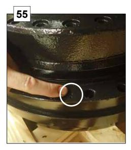
Remove the seal from the slewing bearing.
