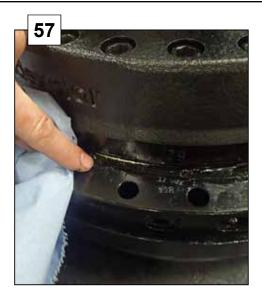
Position the seal with the "lip" against the slewing bearing.
