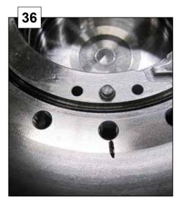
Position the motor according to the aligned marks.
