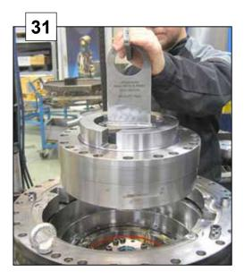
Remove the o-ring in stator upper.
