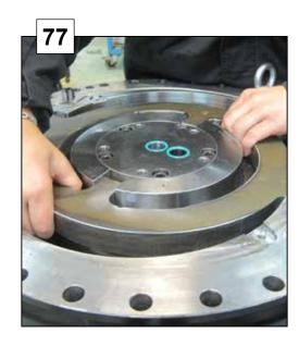
Remove 3 pcs of M8x50 screws in the lower link.
