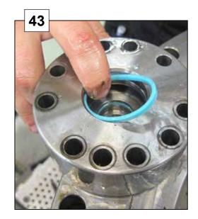
Remove 2 pcs of o-rings at the grapple channels in stator upper.
