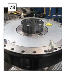
Remove the manifold block by loosen 5 pcs of M12 screws.
