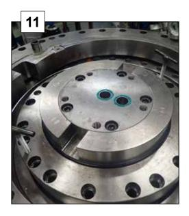
Remove the stator plate lower.
