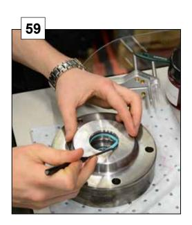
Make a mark on the outside of the rotator shaft and the block lower where the dowel pins are positioned. The block lower is in the end position when the upper surface has the same level as the surface of the rotator shaft.
