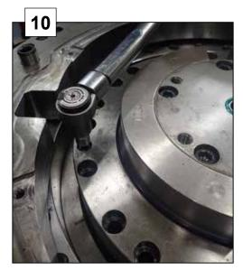
Remove stator plate lower.
