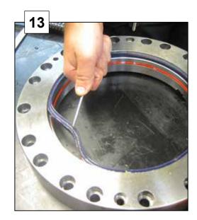
Remove the seal in stator plate lower.
