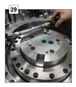
Disassamble the plugs/fittings from the grapple- and rotation inlets. That will make it easier to lift the motor off.
