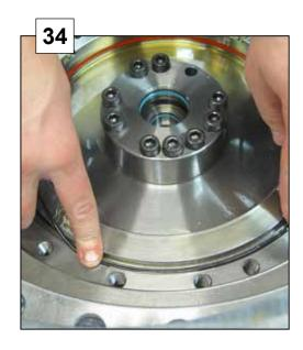
Remove the seal in stator upper.
