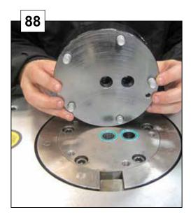
Assemble the manifold block with 6 pcs of M12 screws to a torque of 120 Nm.
