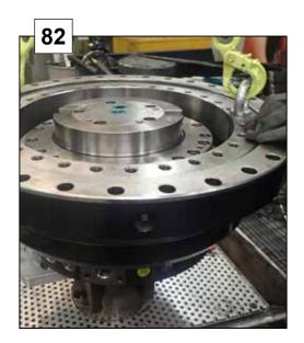
Assemble the 20 pcs of M12x110 screws in the slewing bearing.
