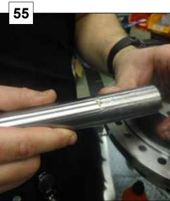
Assemble the internal tube inside of the outer tube. Press down the internal tube by hand till a "click" sound can be heard.
