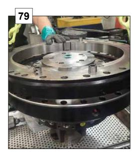
Remove the 20 pcs of M12x110 screws from the slewing bearing.
