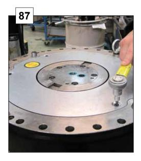
Make sure the grapple channels in the manifold block aligns with the channels in block lower.
