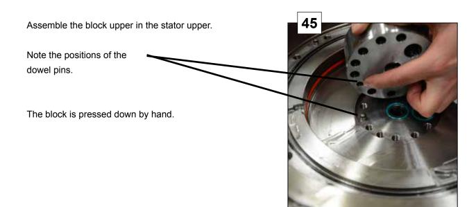
Assemble 9 pcs of M10x60 in block upper. Crosswise tightening to a torque of 60 Nm.
