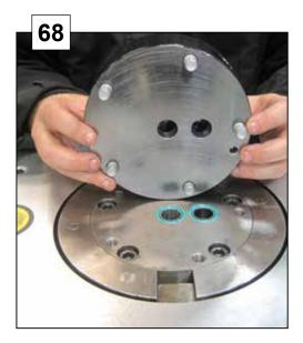
Assemble the manifold block with 6 pcs of M12 screws to a torque of 120 Nm.
