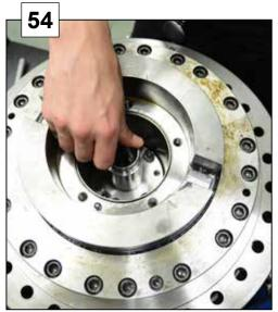
Grease the internal tube.
