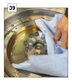
Remove the block upper by loosen 9 pcs of M10x60 screws.
