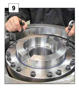
Remove 2 pcs of M8x65 screws - holding the motor parts together.
