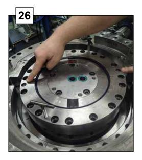
Knock - with care - the stator plate lower the whole way down with a plastic mallet.
