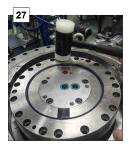
Stator plate lower is in the end position when the wiper seal is visible.
