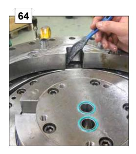
Grease the recesses for the transmission on the rotator shaft.
