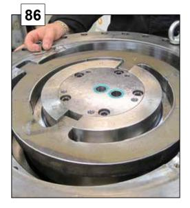
Assemble the bottom plate with 4 pcs of M8x12 screws to a torque of 16 Nm.
