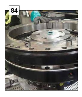
Assemble 3 pcs of M8x50 in the lower link. Torque 33 Nm.
