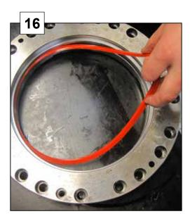
Assemble a new wiper seal (not for c-models).
