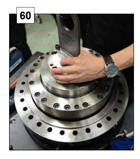
Assemble 5 pcs of M12x45 screws. Crosswise tightening to a torque of 120 Nm.
