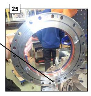
Make sure that the holes in stator plate lower aligns with the two holes for M8x65 screws in the stator frame.
