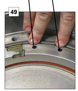
To make the reassembly of the motor easier, make a mark on the outside of the stator frame where the dowel pins are positioned.
