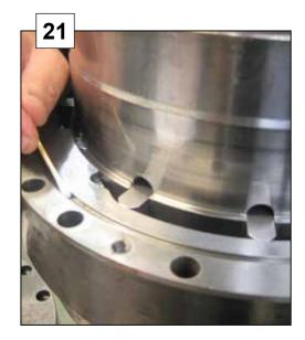
Lubricate the seal seat with oil.
