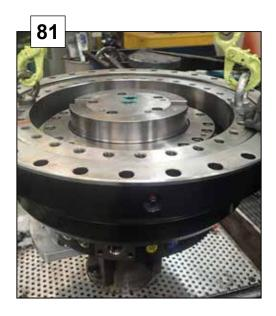
Assemble a new slewing bearing.
