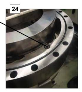
Assemble stator plate lower on the motor part.
