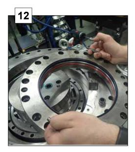
If needed remove the wiper seal (only if it has a damage). The wiper seal is ordered separately, is not part of the seal kit.
