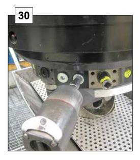
Lift the motor off from stator upper.
