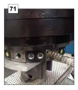
NOTE! The grapple outlets (G, G0) on the manifold block have to be sealed by steel plugs before testing!
