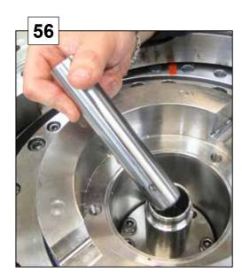
Grease the edges of the outer tube and the internal tube.
