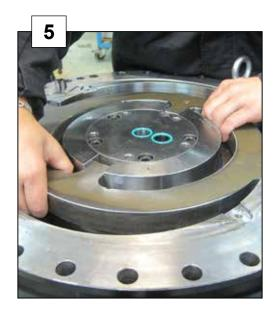
Remove 5 pcs of M12x45 screws in block lower.
