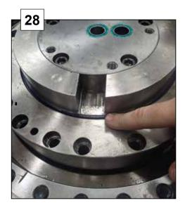
Assemble 2 pcs of M8x65 screws holding the motor parts together.
