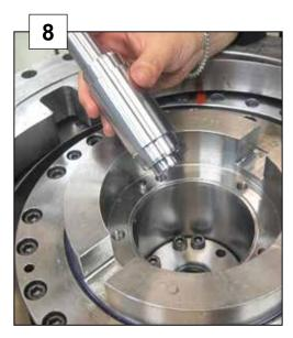
Remove 20 pcs of M12x110 screws to loosen the motor part.
