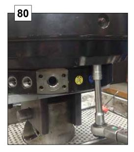
Lift the slewing bearing.
